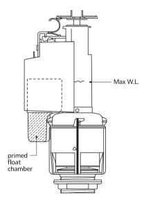
To maintain correct short flush volumes in hot climates, it may be necessary to carry out this procedure on a regular basis due to evaporation.
