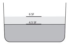
Water lines marked 4.5 SF and 6 SF are indicating full flush volumes in litres. These waterlines are for use with either a SF or DF "Fast Part" branded push button valve.
