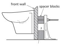
where there is a void between the pan and the bracket this must be filled with spacer blocks (as shown) or equivalent
