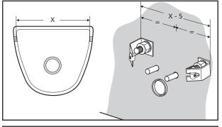
3. Position sliders correct distance from wall.
