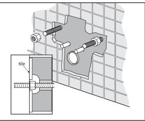
Fit brackets to support bolts (cut to length as necessary), using fixings supplied.
