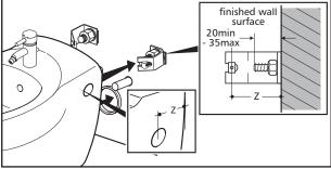
4. Fit bidet and secure with fixings provided.
