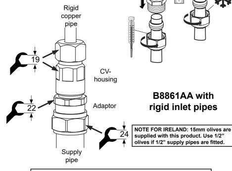
RESTORE SUPPLIES & CHECK ALL JOINTS FOR LEAKS
