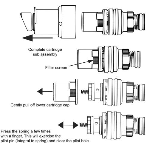
Before reassembling the cartridge cap, make sure that the filter screen is clean (slides out from inside of cap). When reassembling, take care to ensure the spring is straight & locates correctly into the boss at the bottom of the cap moulding.
