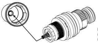
Finally refit the cartridge back into the brass housing, refit into mixer, reset the run-time & fit the handle.
