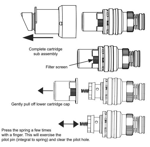
Before reassembling the cartridge cap, make sure that the filter screen is clean (slides out from inside of cap). When reassembling, take care to ensure the spring is straight & locates correctly into the boss at the bottom of the cap moulding.
