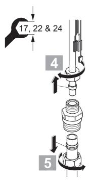
**4. To fit inlet adaptor:** Slip the small compression nut & olive onto the Ø10mm inlet pipe. Push the adaptor onto the inlet pipe up to the shoulder. Slide the olive up to the adaptor & tighten the compression nut
