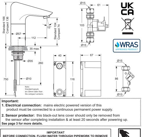
BEFORE CONNECTION, FLUSH WATER THROUGH PIPEWORK TO REMO ALL DEBRIS ETC. WHICH COULD DAMAGE THE VALVE MECHANISM
