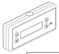
The programming unit should be held pointing towards the sensor at distance of approx. 100mm.
