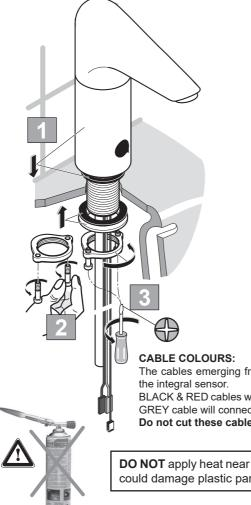
Feed the inlet pipe & cables through basin hole. The cables are protected by the black corrugated plastic tubing (split). Locate the spout tail into the basin hole. Allow the spout to rest on the basin seated on the rubber washer. Refit the corrugated tube if it slips off the cables.
