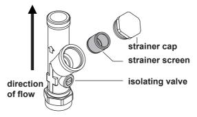
When the isolator screw slot is parallel to the valve body, the valve is open & permits water to flow. To close the valve, rotate the isolator screw 90°.
