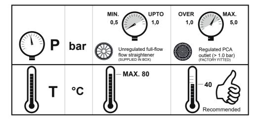
These products are factory fitted with a regulated PCA outlet, this outlet will function correctly at pressures greater than 1 bar. For lower pressure systems fit the unregulated flow straightener supplied. For more outlet details see section 8
