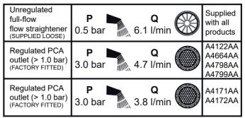
Note: The 3.8 l/min & 4.7 l/min aerators are supplied as shown above, but can be used in any of the product codes.
