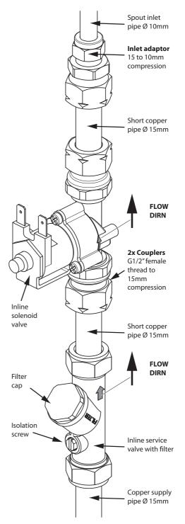
**5.** To fit inlet adaptor cont: Slip the larger compression nut & olive onto a short length of Ø15mm supply pipe. Push the supply pipe into the adaptor up to the shoulder. Slide the olive up to the adaptor & tighten the compression nut with a 24mm A/F spanner. Hold the adaptor steady with a 22mm A/F spanner.
