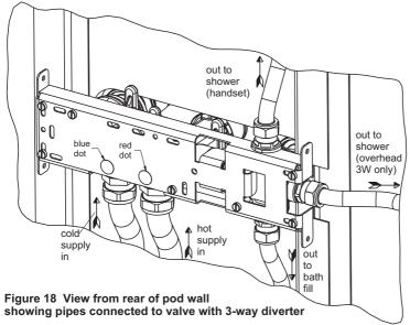
Pipe work connections should be made as shown. Red and blue dots on the bracket indicate hot and cold supply connections respectively. The outlets can be plumbed as shown. There will be either 2 or 3 outlets depending on the product being installed (2 or 3 way diverter). This completes the installation from the rear of the pod wall.
