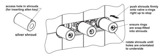
Figure 21 View of valve from inside of pod with shrouds fitted
