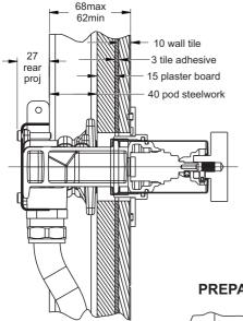
Figure 5 Section through typical pod wall
