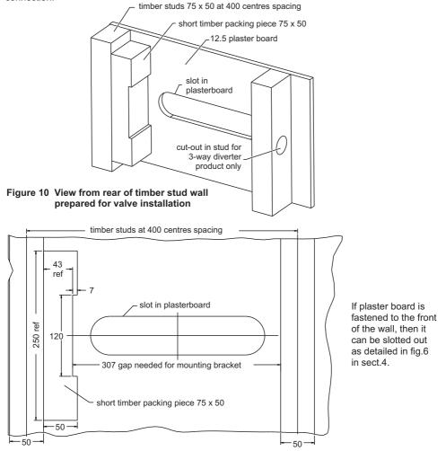
Figure 11 View from rear of timber stud wall showing dimensions
