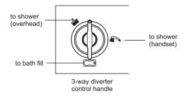
Figure 33 Quick reference to functions for 3-way diverter
