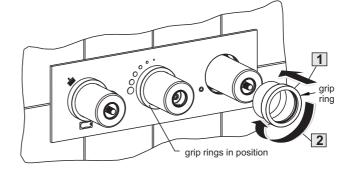
Figure 26 View of valve from inside of pod - grip rings being fitted
