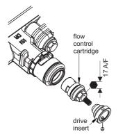
The flow control cartridge is the central control. This controls the volume of water flowing from the built-in valve.
