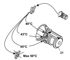
Figure 39 Adjusting the temperature limit stop
