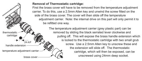
Figure 34 Thermostatic cartridge removal
