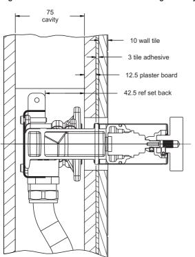
The exact mounting depth is dependent on the thickness of plaster board and tiles being used. The 42.5 dimension is given here as a guideline only.
