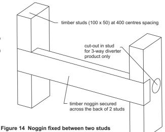
The valve can now be fastened to the noggin using 4 suitable wood screws.
