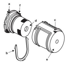
Figure 38 Temperature adjustment carrier exploded
