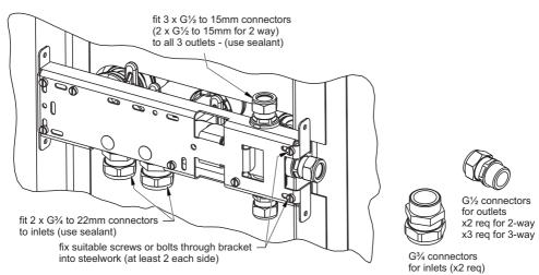
Figure 17 View from rear of pod wall with connectors fitted
