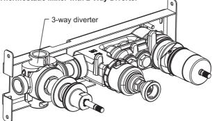
Figure 3 Thermostatic Mixer Valve body with 3-Way Diverter complete with mounting bracket
