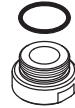
A6256AA Universal filter adaptor. Replaces the Armitage Bioguard outlet to permit attachment of an outlet filter. Threaded M24x1 (internal).
