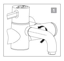
To remove the spout: gently rotate the end of the spout anticlockwise by 90°.
