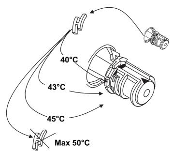
Figure 13 Adjusting the temperature limit stop
