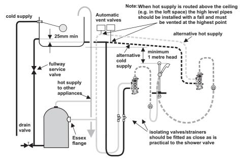
Figure 5 Recommended system layout for gravity applications
