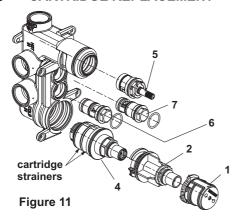
Servicing the thermostatic valve is simple as all working parts are in the replaceable cartridges.
