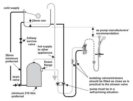
Figure 6 Recommended pumped system layout
