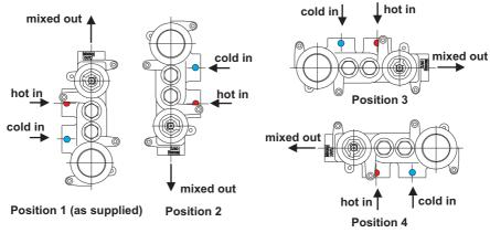
Figure 8 Preferred installation orientation
