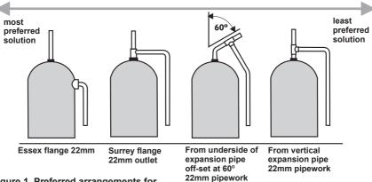
Figure 1 Preferred arrangements for cylinder tapping
