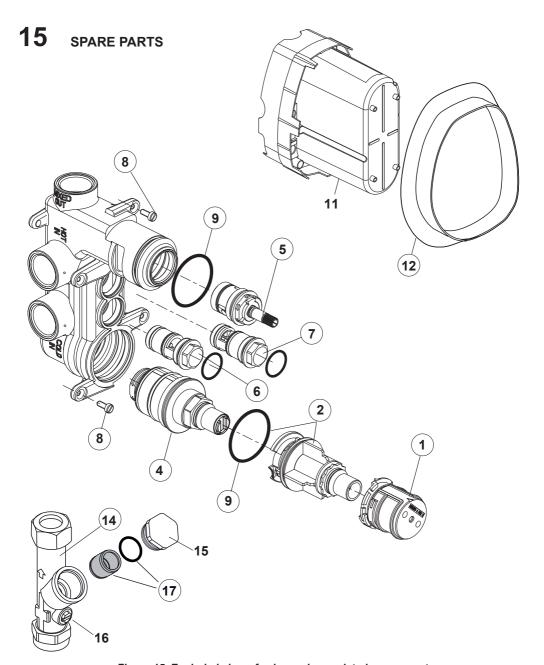
Figure 15 Exploded view of valve and associated components
