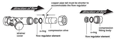
Figure 2 Fitting the regulator in the downstream end of the iso' valve/strainer
