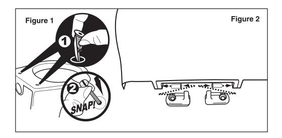
Insert the sprung retainers into the pan, before snapping into place with a screw. (Figure 1)
