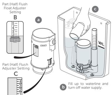
The Part Flush volume should be no more than 2/3rds of the full flush volume.
