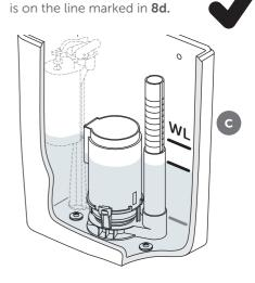
Repeat flush and adjustment until the part flush residual water level
