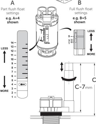
**C** is the overflow tube height measured from the base of the tank. Subtract 7 if measuring from the base of plastic cadge without the seal.
