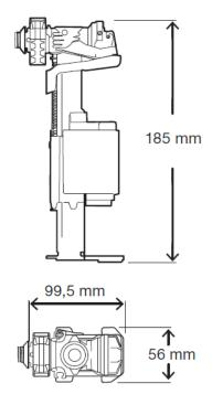
(measurements in mm)
