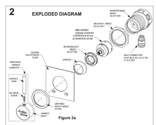
Check that all the parts shown above are available. The chromed grip ring and square escutcheon plate & handle parts are will be packaged separately. The grip ring will have two o-rings fitted to it.
