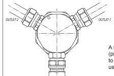
Fig 5a. Rear view of diverter showing couplers fitted.
